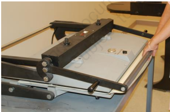
A heat press is used to flatten the document in order to obtain the best initial capture.
