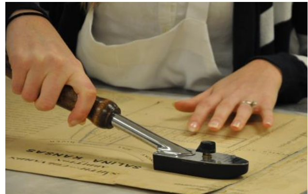
A tacking iron, a specialized tool with temperature controls, flattens standard sized documents.
